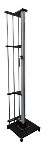
USED TO TEST IMPACT RESISTANCE
